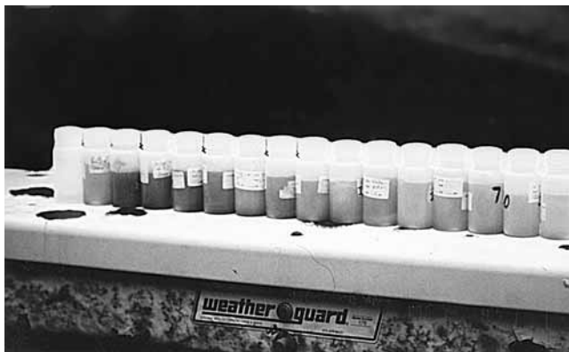
Figure 1—A time sequenced display of tile drain samples showing rapid contaminant delivery (first on left = pre-irrigation, followed by left to right = 35 min through 330 min samples after the start of irrigation).
